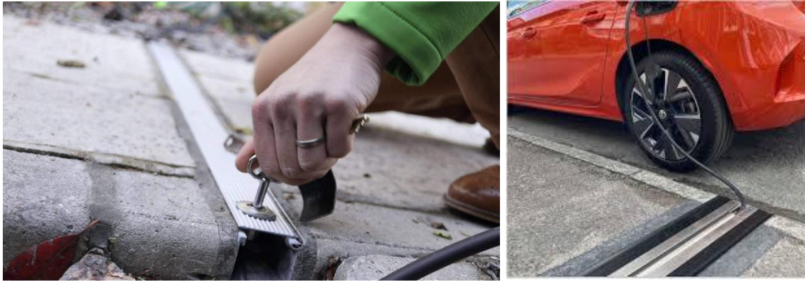
Figure 8 Examples of cross pavement charging solutions:
