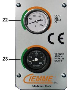
Always check the diathermic oil temperature before opening the lid and carrying out the discharge. Open the lid and carry out the residuum discharge with the greatest care in relation to the residuum temperature.
