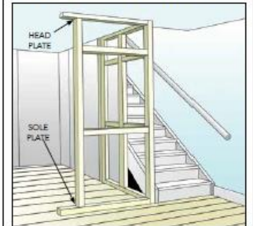
Diagram 1: Example of fire resisting partitions (half hour fire resistance) The studding framework should be 75mm x 50mm and should be securely fixed where it joins floor, adjacent walls and true ceilings.
